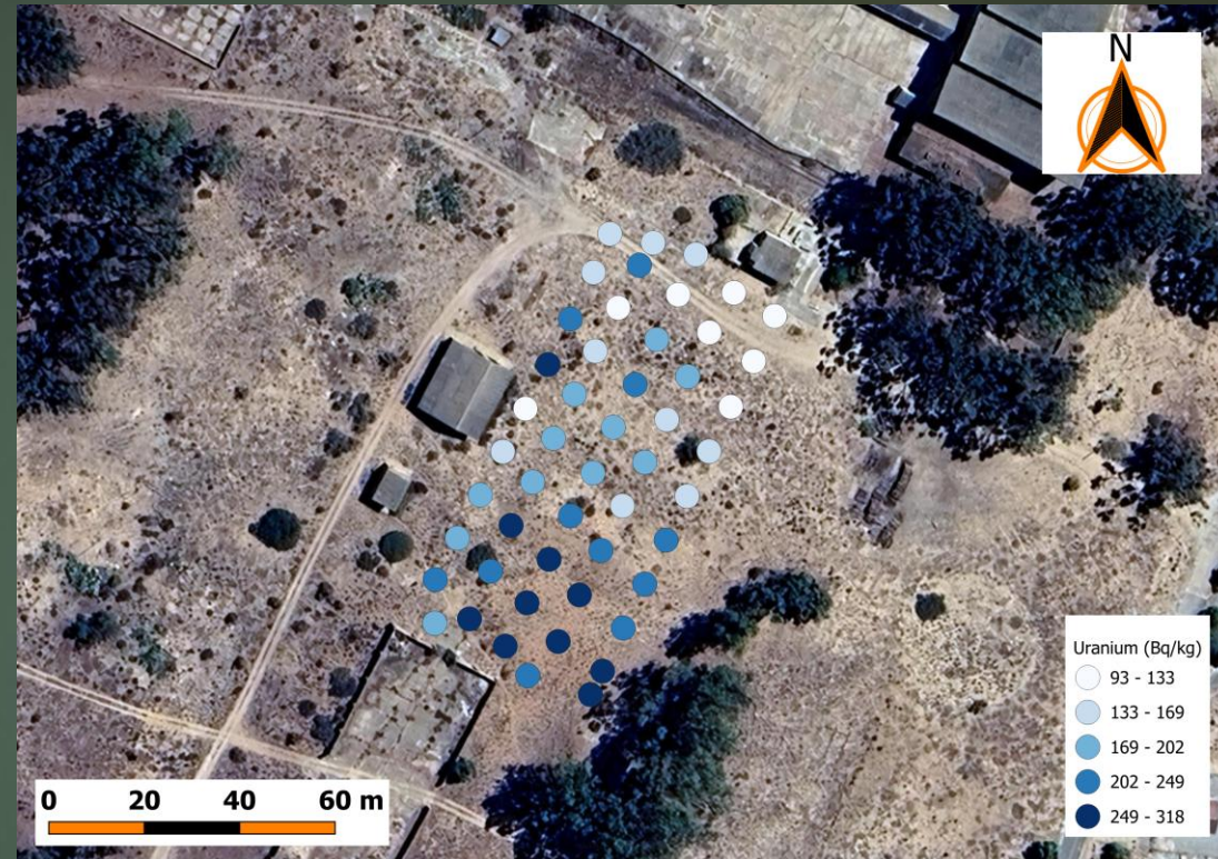
Figure 5: Distribution of uranium concentrations (Bq/kg) measured at discrete sampling points across the site. Each circle represents a sampling location, with colors corresponding to uranium activity levels ranging from 93 to 318 Bq/kg.
