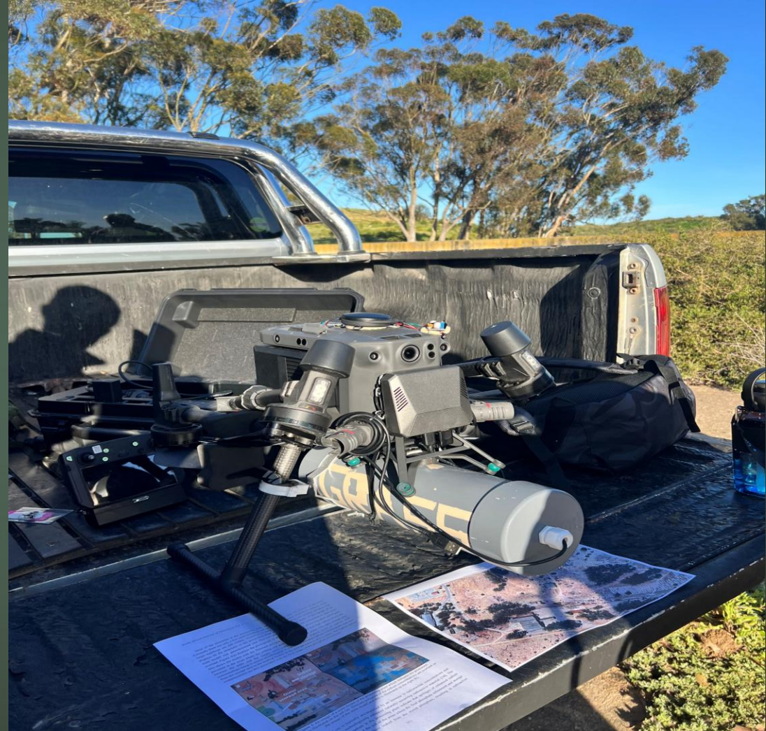
Figure 2: GRASS UAV System used for the radiometric measurements.
