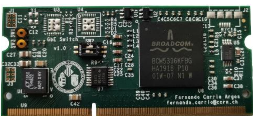
Tile GbE PCB populated with components
