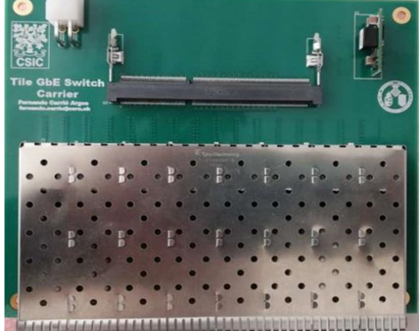
Tile GbE motherboard to insert Switch
